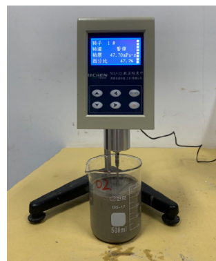
图11 水泥浆液动力黏度测试图 Fig.11 Schematic diagram of dynamic viscosity test of cement slurry
